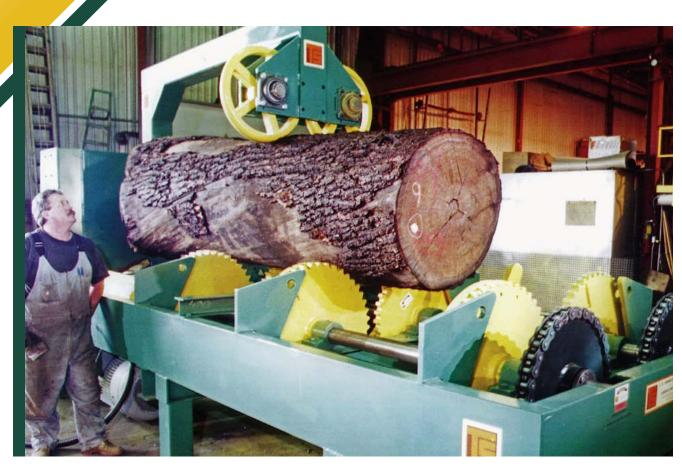
TS Manufacturing Log Reducers are the ideal solution to log butt flare and its resulting inefficiencies throughout the line. Whether you're looking for reduced maintenance on your debarker head or veneer knives, or simply wish to solve material flow issues associated with large slabs, a Log Reducer from TS is an excellent solution.
