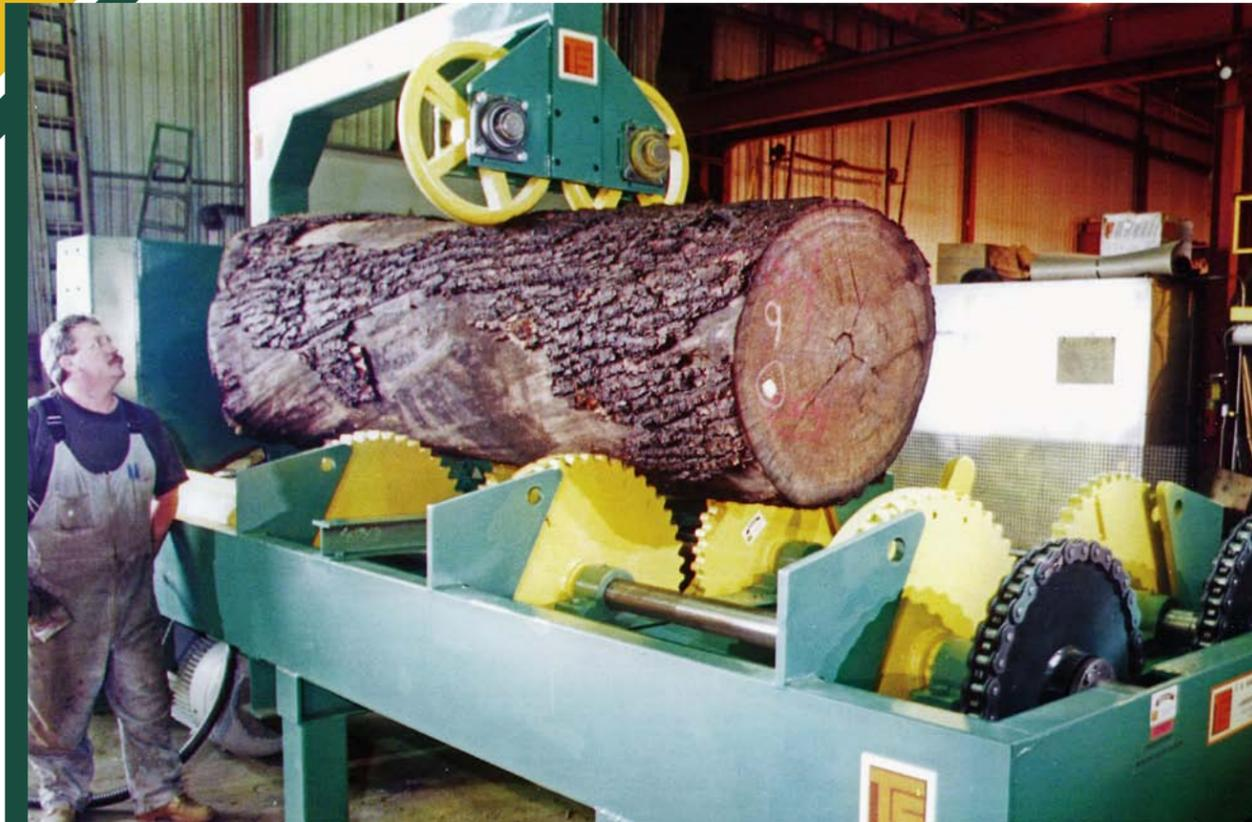
**TS Manufacturing Log Reducers are the ideal solution to log butt flare and its resulting inefficiencies throughout the line.** Whether you're looking for reduced maintenance on your debarker head or veneer knives, or simply wish to solve material flow issues associated with large slabs, a Log Reducer from TS is an excellent solution.
